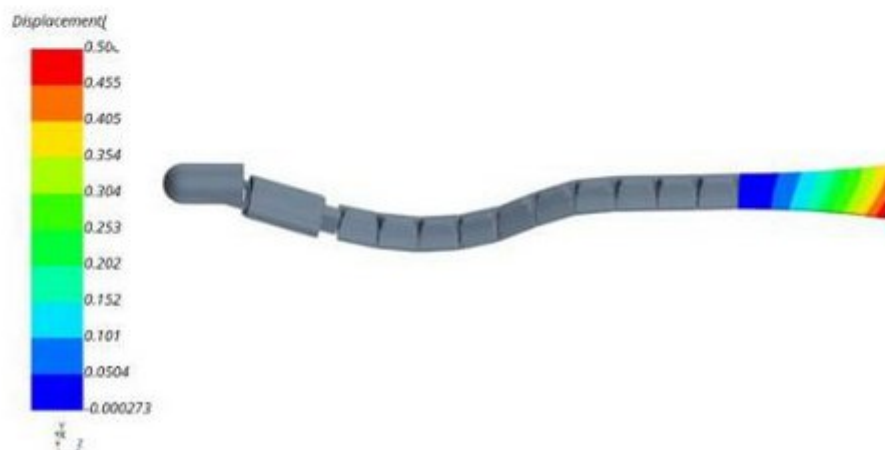
(b) EEL tail exhibiting low flexibility with peak solid displacement less than 1 mm
