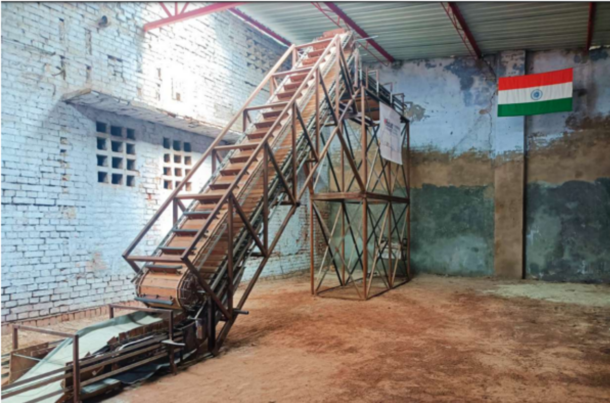
Gravity storage mechanism Image: Baud Resources
